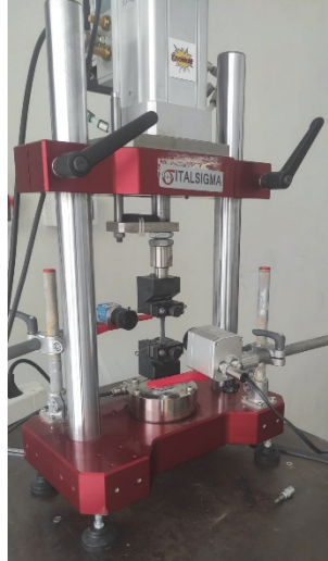
Figure 2: Fast Fatigue Machine with IRtech XT IR camera and Basler camera acA2440-35uc for DIC.
