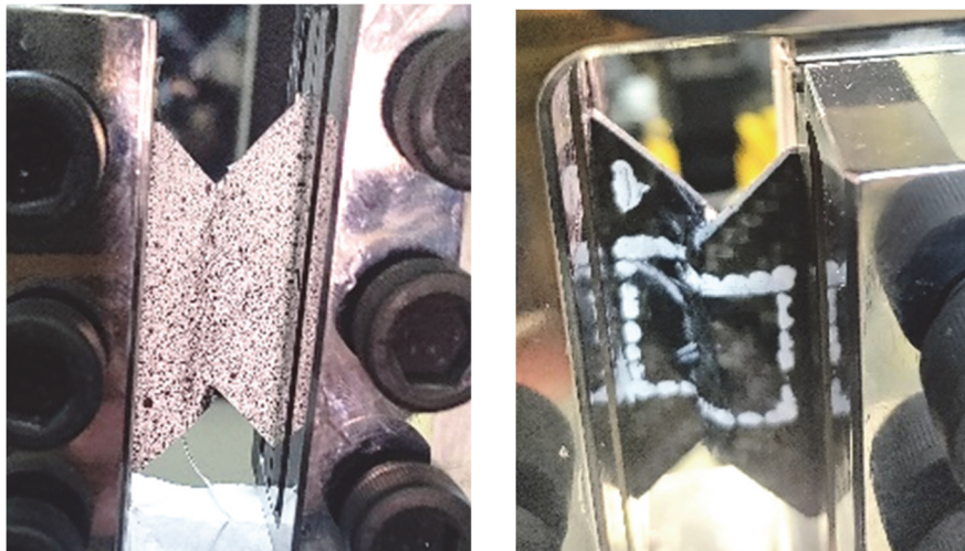
Figure 7: Typical failure modes.
