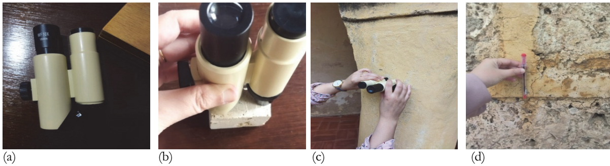
Figure A2-14: (a) the crackmeter from MATEST, (b) tested samples, before and after durability tests (c, d) the use of the crackmeter in the measurement of cracks development in the gallery support and the jointing mortar.
