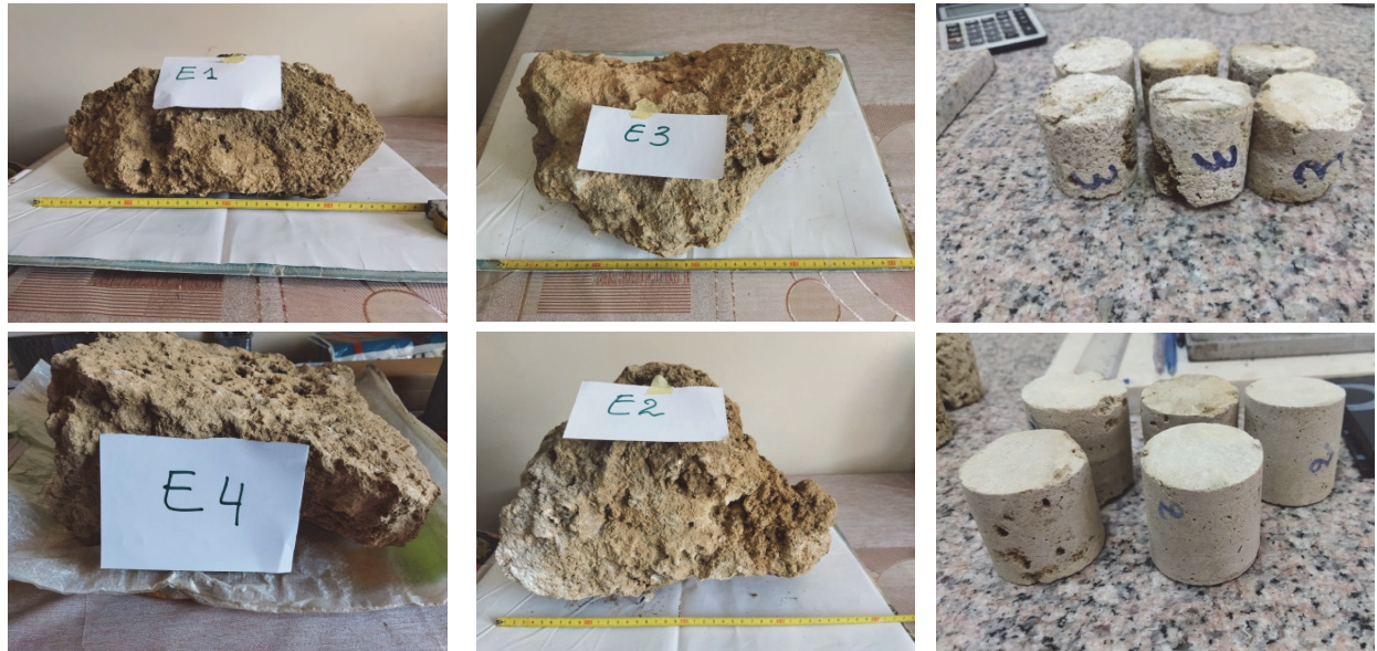
Figure 5: Stone samples and extracted cylindrical specimens.
