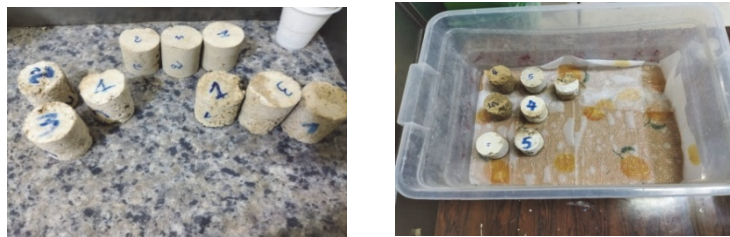
Figure A2-7: Water absorption by capillarity test.
