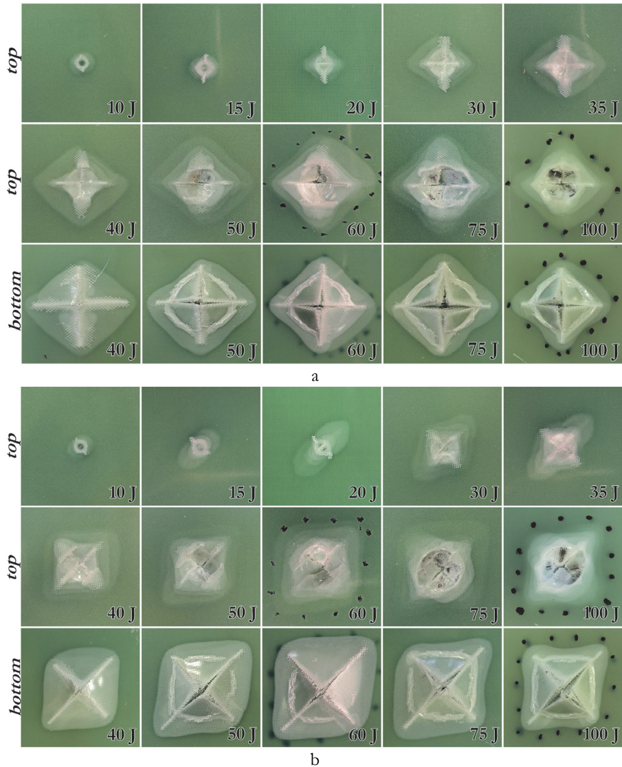
Figure 4: Images of specimens with the reinforcement schemes [0/90]_n (a) and [\pm 45]_n (b) after impacts
