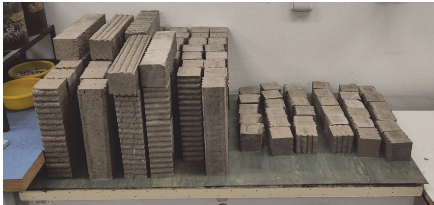
Figure 5: Extracted sub-sections of walls from the 3D printed test specimens.
