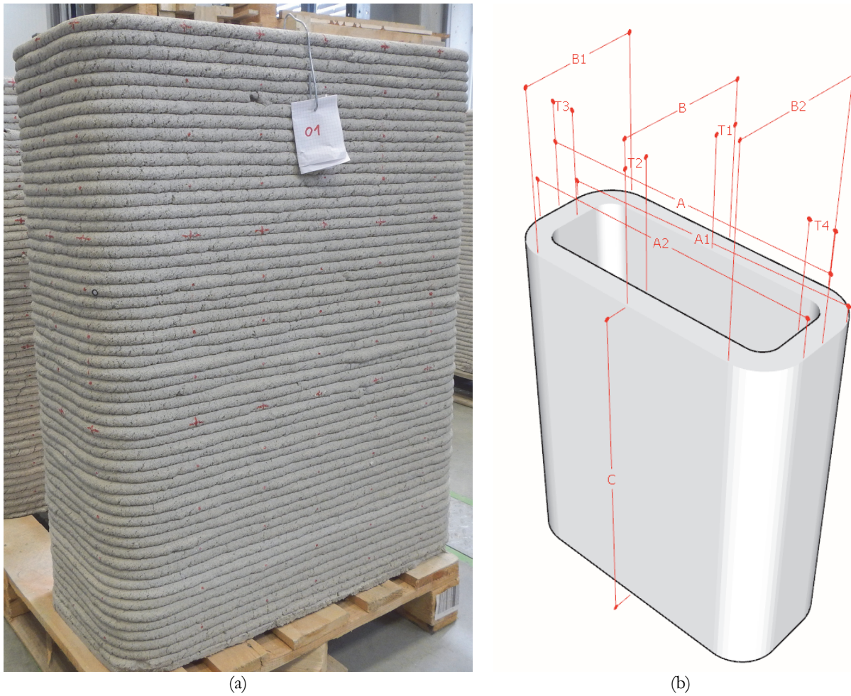
Figure 1: Illustration of tested specimens (a) and the main measured dimensions (b)
