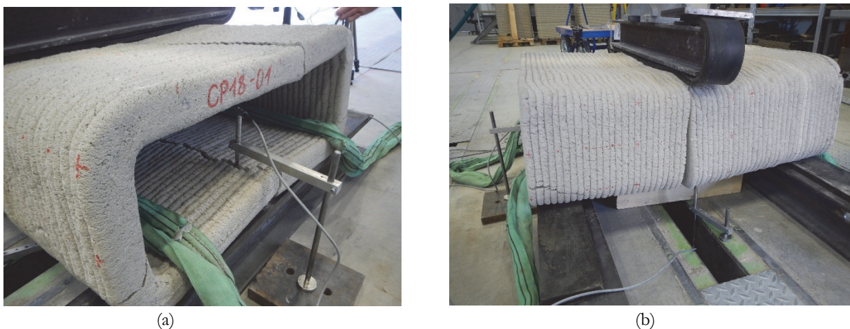
Figure 3: a) Fractured specimen CP18-01; b) Fractured specimen CP18-02.
