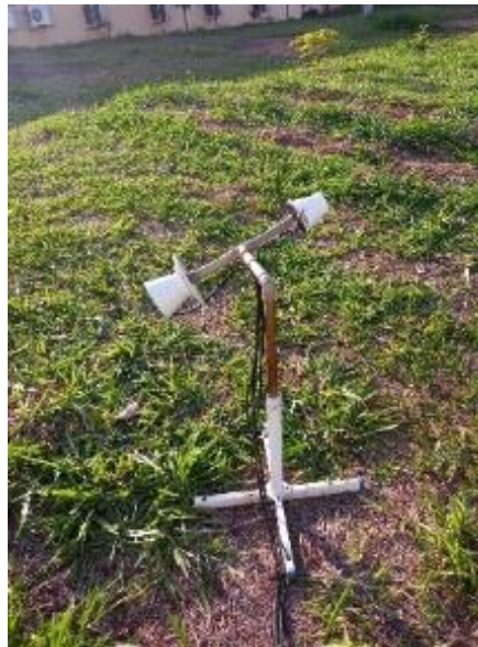
Fig. 8 Radiometers for incident and reflected radiation
