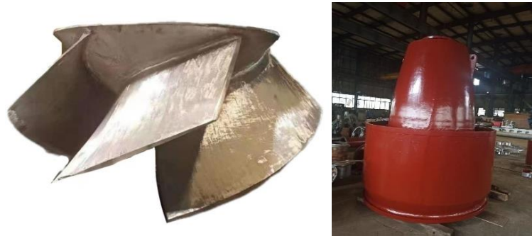
Fig. 17 Field component schematics: Impeller (left) and painted guide vane body (right)
