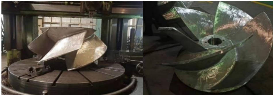
Fig. 5 Model of a mixed-flow pump's impeller
