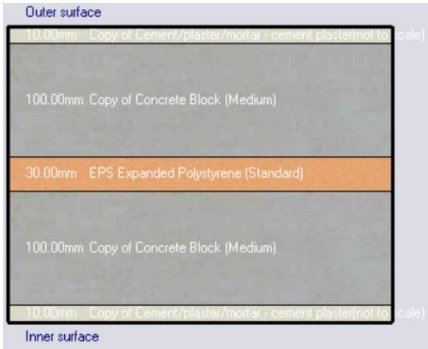
Figure 4. Building envelope insulation
