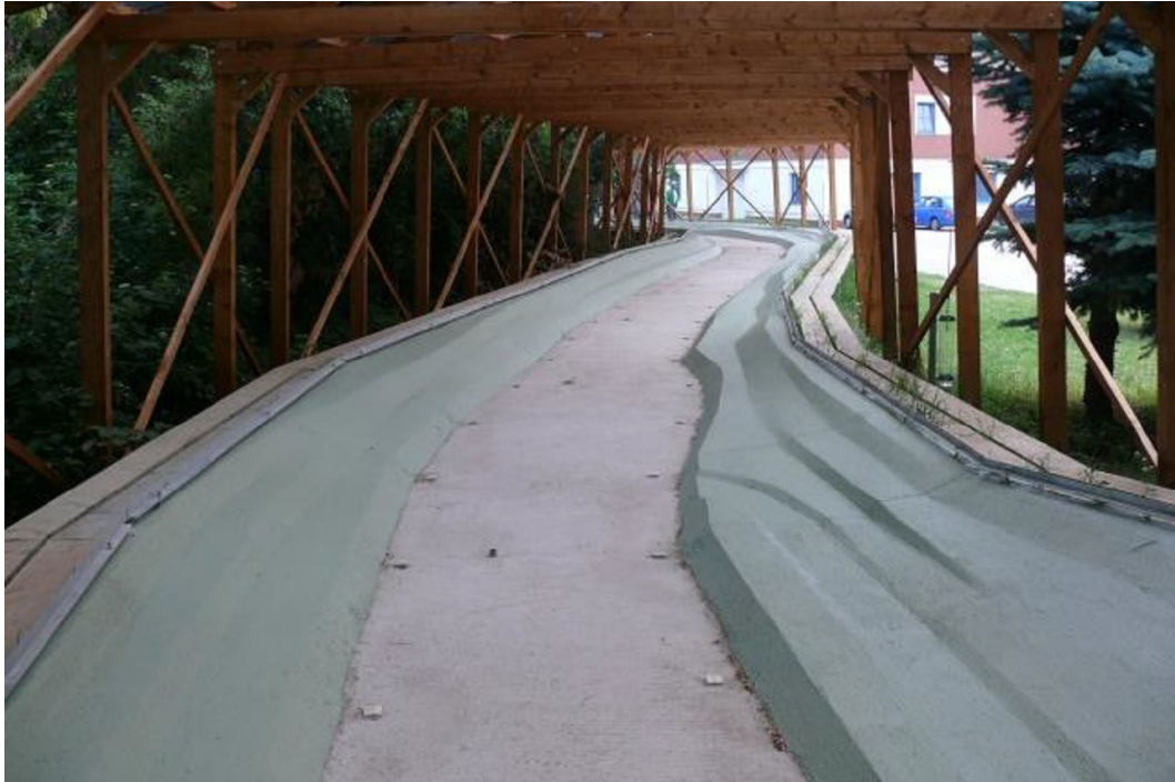
Figure 2: River model in reality (sand riverbed and concrete banks)
