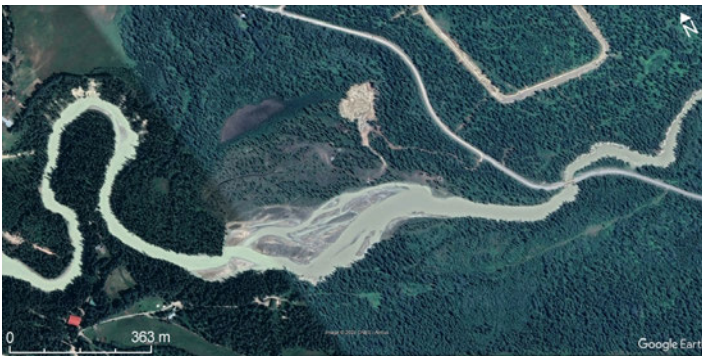
Figure 31. Example of a sinuous, single-threaded river transitioning to a multithreaded river and back to a sinuous, single-threaded river. Flow is toward the left. Blaeberry River, British Columbia (51.4265°N., -117.0507°W.). Imagery date: October 11, 2021, Google Earth.
