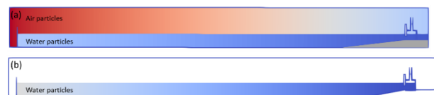
Figure 1 - Numerical wave flume set up of (a) multiphase and (b) single-phase with colors indicating the particles generated.
