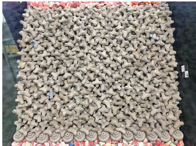
Figure 6. Detail of the ACCROPODE™ II armour placement
