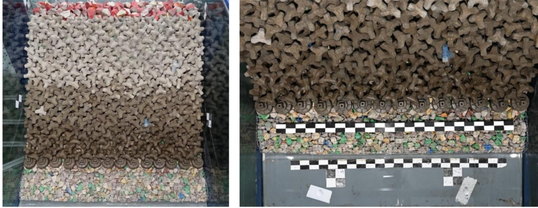
Figure 8. Example of perpendicular photo of the armour layer (left) and vertical photo of the toe berm (right)
