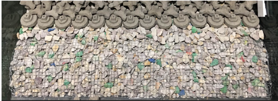
Figure 5. Rigid wire mesh applied to the rock berm supporting the ACCROBERM™ I units
