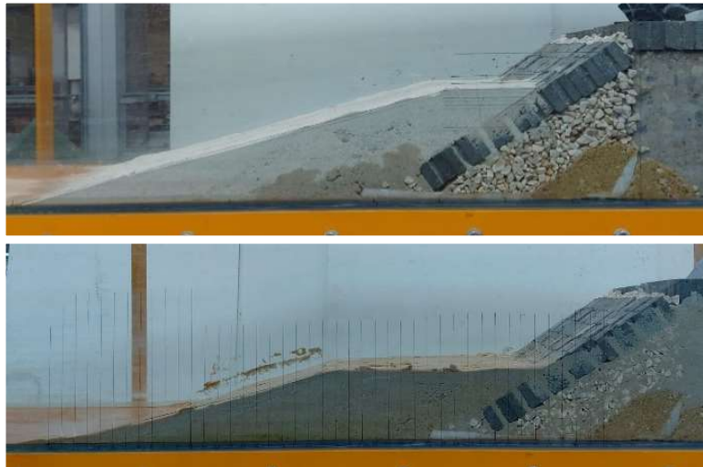
Figure 2. Beach profiles tested: top) 15cm initial emerged berm level; bottom) 10cm initial submerged berm level (adopted from Pires, 2024).
