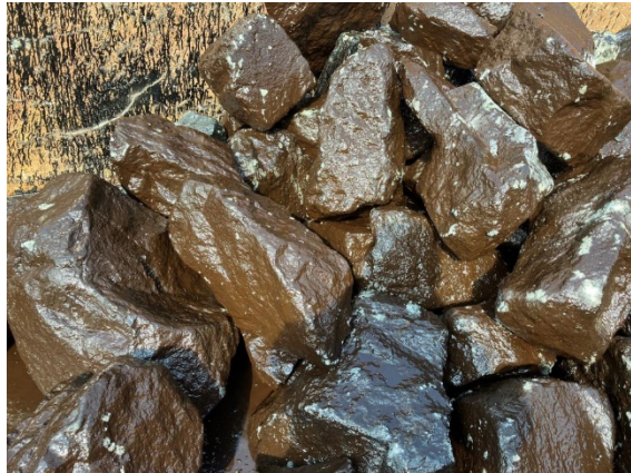
Figure 19. Pretreated armour stone with a bitumen layer.
