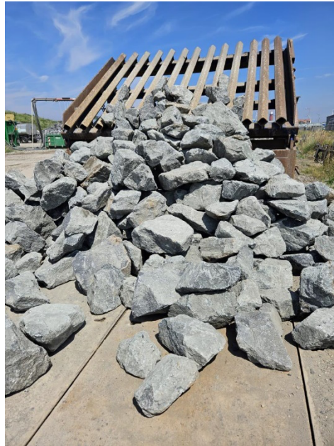
Figure 17. Process of filtering out the fine fractions of the armour stone.
