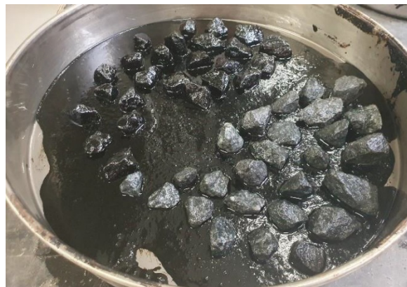
Figure 15. Queensland test with left above the pretreated armour stone and right under the 'clean' armour stone.
