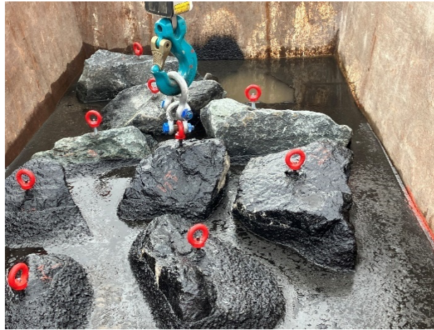
Figure 16. Full scale pulling test with pretreated and not pretreated stones.
