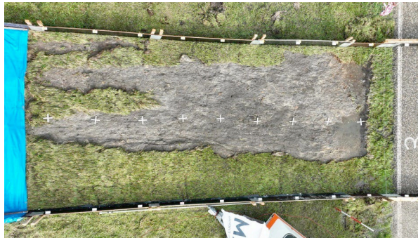
Figure 11. Almost complete erosion of the transplanted grass sod (5 cm thick), but then similar erosion of the underlying clay of the rounded geometrical transition, showing similar loads over the transition.
