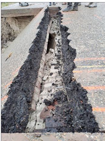
Figure 16. Classical mechanical failure after forced undermining up to 2.9 m.
