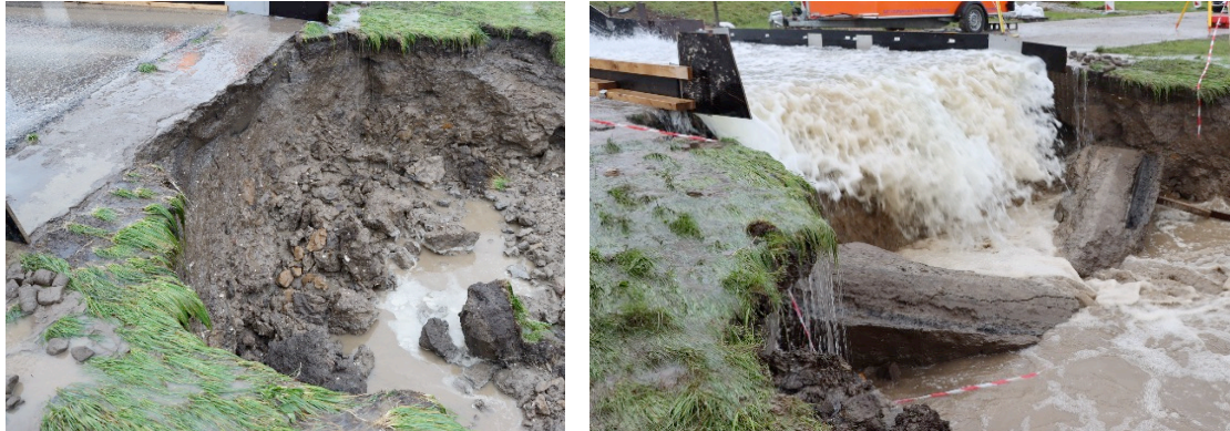
Figure 13. Cliff erosion test. The 1 m wide (boulder clay with grass cover) fails after 45 minutes (left). The 0.7 m wide Mixed-in-place block fails 30 minutes later (right).
