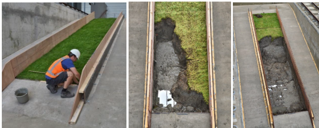
Figure 8 Model set-up of test series K1 with clay type Lauwersmeerdijk with the erosion process halfway the test series and at the end of the test series.
