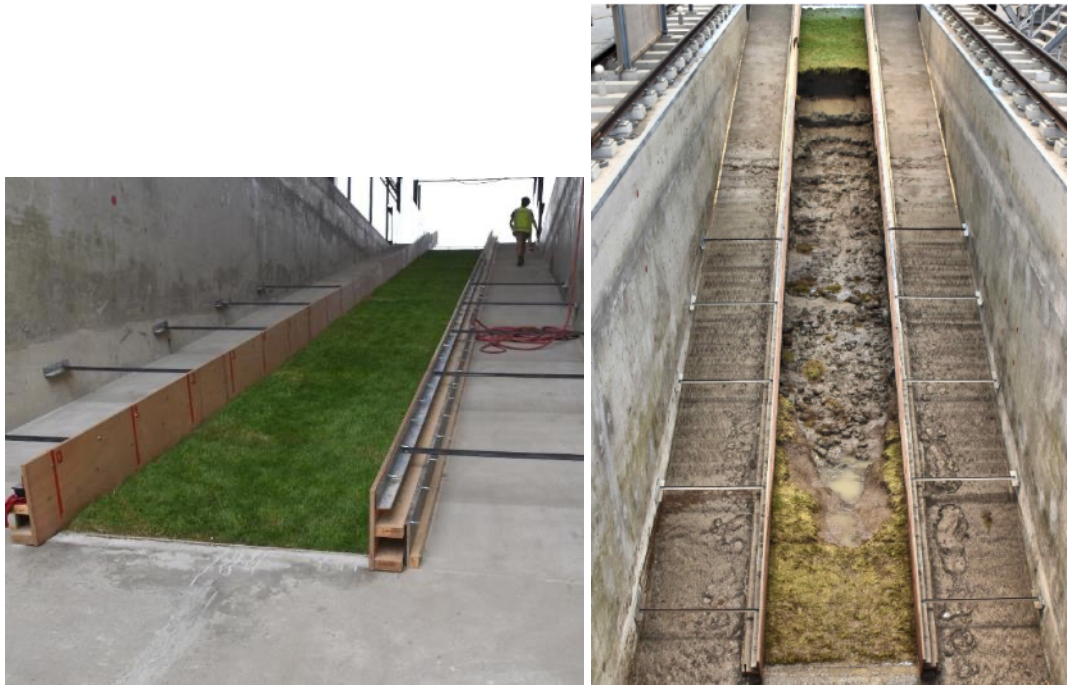
Figure 10 The model set-up of test series EK1 and the final erosion hole of the measurement campaign Dubbele Dijk.
