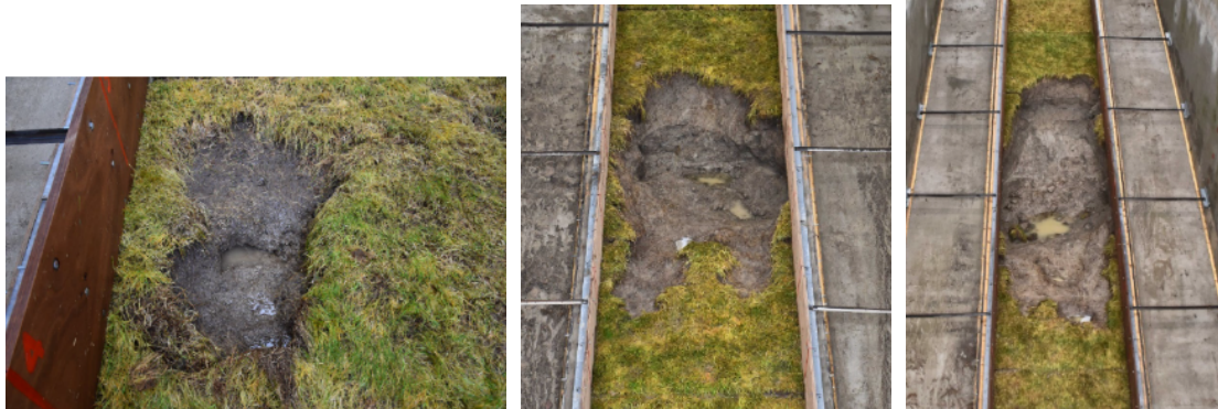
Figure 13 Photos of the three phases of the erosion process during test series EK2. Phase 0: grass cover failure with a damage of 28 cm depth. Phase 1: deepening of the erosion hole to a depth of about 0.6 m and the start of a small cliff forming. Phase 2: cliff erosion and formation of a terrace.
