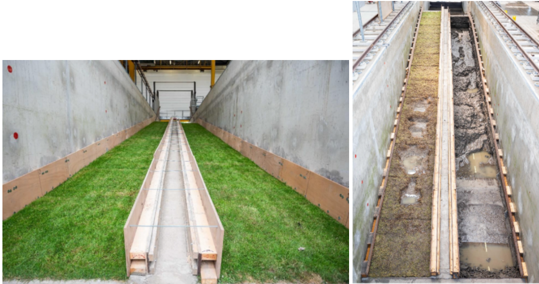
Figure 9 The Wide Green Dike model set-up with two clay types: Blija2021 (left side) and Dollarddijk (right side) at the start and end of test series B2
