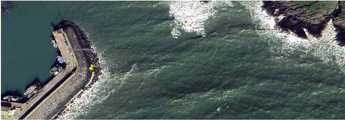
Figure 16. Ardglass Breakwater: mach-stem waves were experience on the trailing leg during model studies
