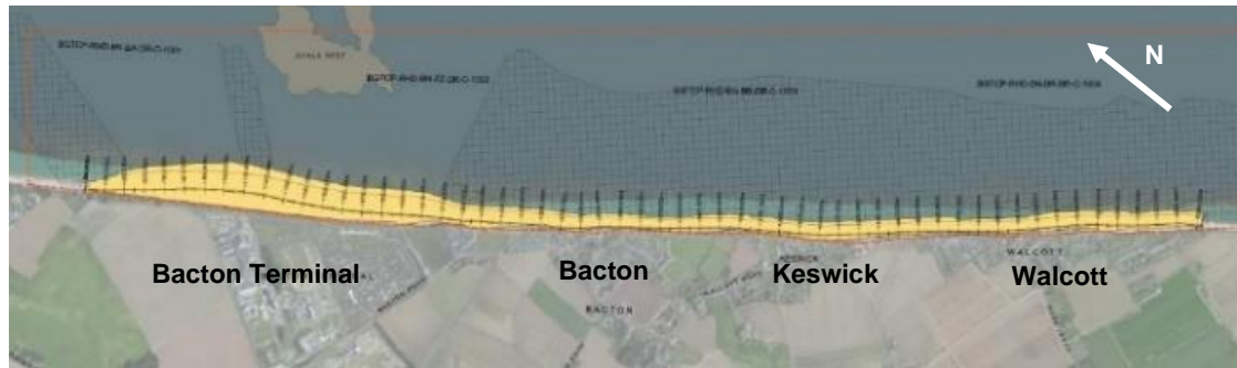
Figure 1: Impression of the implemented Bacton Sandscaping Scheme, stretching approximately 2km from the Bacton Terminal towards Walcott.
