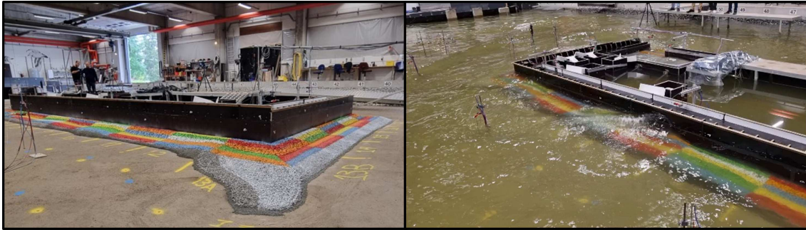
Figure 5: Overview of the 3D experimental set-up, with left the basin without water with distinct colored boxes for different scour protection areas and right a snapshot of wave attack during one of the tests.
