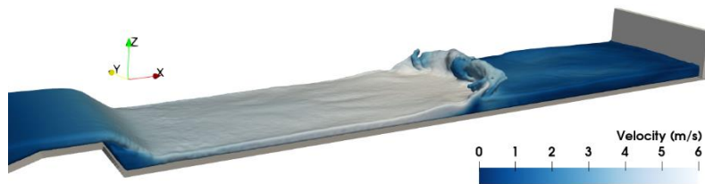
Figure 16. Interaction of second bore leading tip with impounded water, at t = 21 sec.
