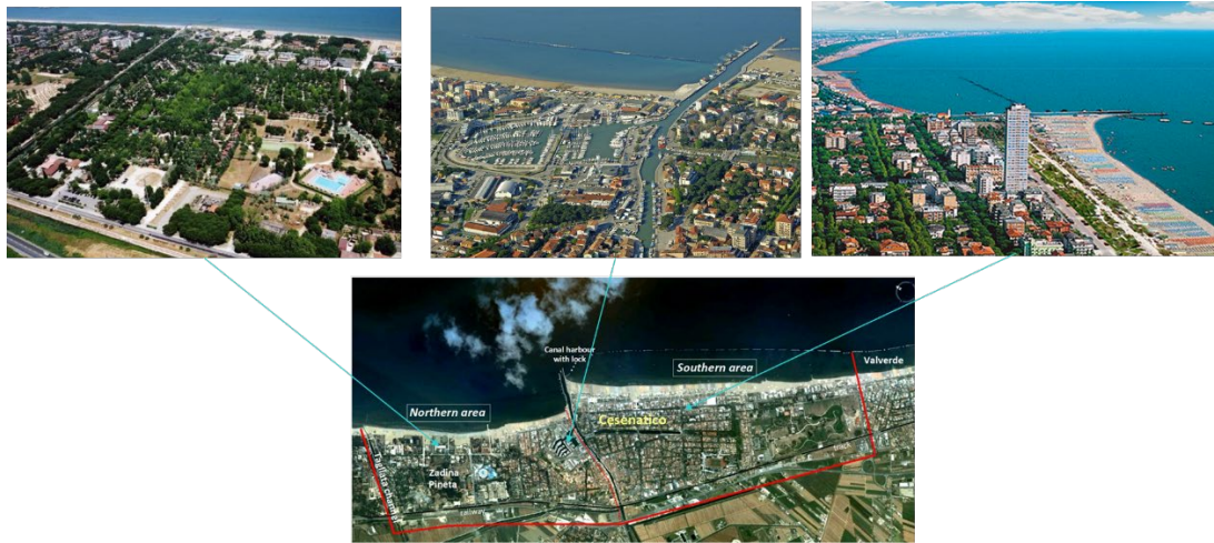
Figure 4. View of Cesenatico i) at the bottom: satellite view with indication of the Northern Area, Southern area and Valverde; ii) top left: view of the Tagliata Channel and of the Northern area; iii) top center: view of the Central area, with the jetties, the marina and the low crested barrier; iv) view of the Southern beach protected by emerged barriers.
