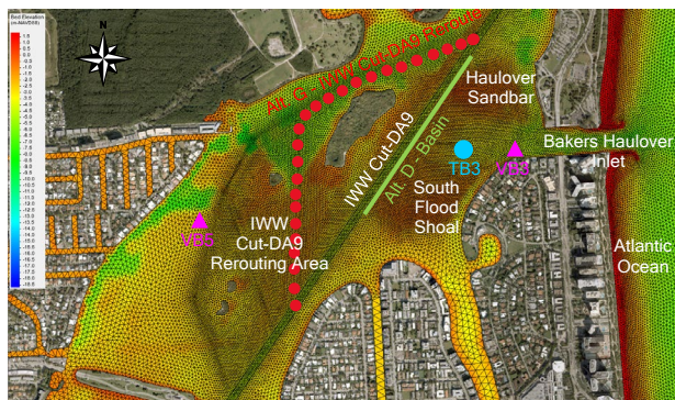
Figure 3 - Model Bed Elevations, Mesh at the Area of Interest, Calibration Stations, and Analyzed Alternatives (Map Data: World Imagery)
