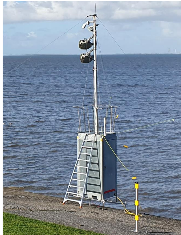
Figure 2 - Laser scanner system on the dike in the Eems-Dollard estuary. From the bottom to the top: laser scanner 1, laser scanner 2, infrared lamp, video camera.
