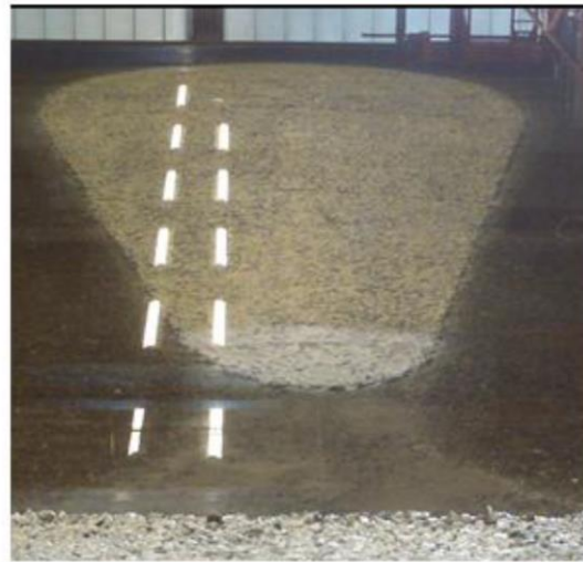
Figure 2 Scaled models of different groin designs. (BAW, 2015)
