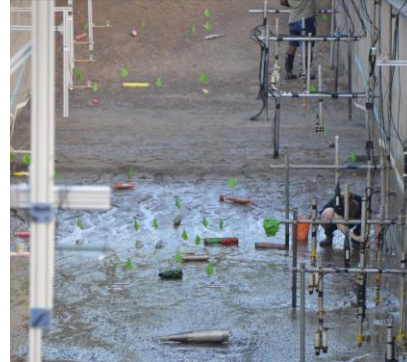
Figure 1 - Image looking onshore showing a drained flume, sensors the right and proud munitions.
