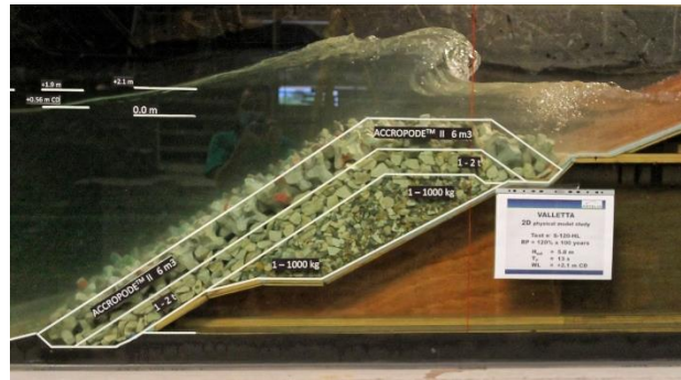
Figure 4 - 2D physical modelling of the detached submerged breakwater
