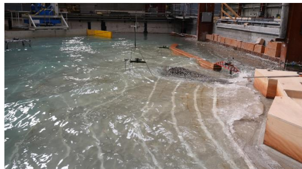
Figure 5 - 3D physical modelling of the outer breakwater
