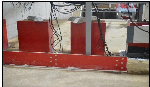
Figure 2 - Test wall section showing two arrays of horizontal mounted pressure transducers. In this picture a failure section is shown to the right of the picture.
