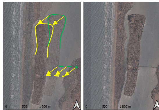
Figure 1 - Example of the geometric correction. On the left an uncorrected single frame and on the right we see a perfect match of the reference image.
