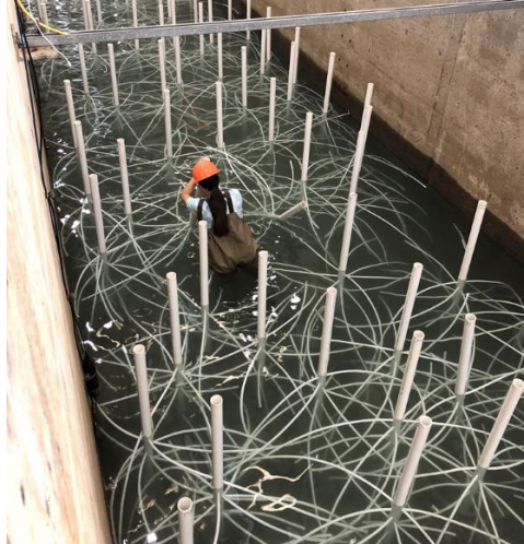
Figure 1 - Photograph of mangrove installation for physical model experiments.
