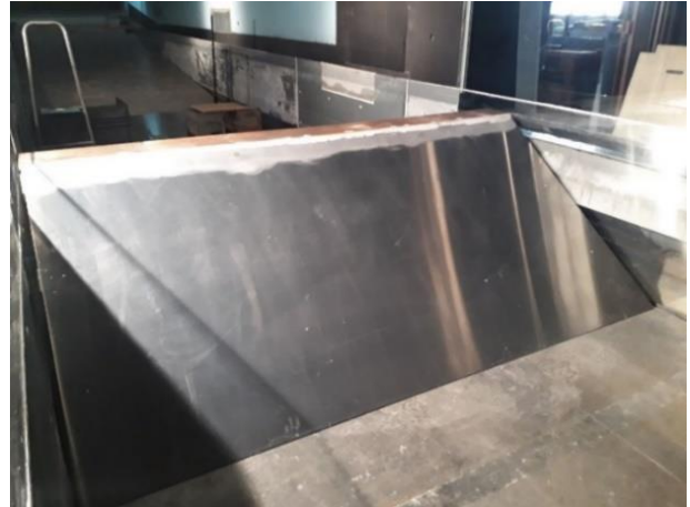
Figure 1 - Picture of the breakwater with a smooth slope.
