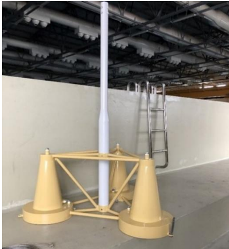
Figure 1 - 1:50 Scaled Semisubmersible Floating Offshore Wind Turbine Platform
