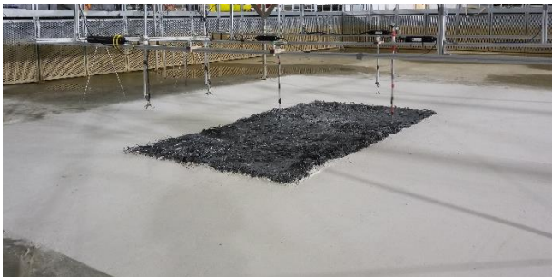
Figure 1 - Experimental setup with an artificial seagrass meadow in compact layout in the 3D-wave basin
