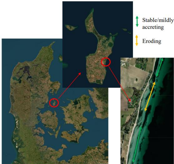
Figure 1: Map showing Denmark as well as a zoom in on the Island of Samsøe and the eastern coast of the island. At the zoom-in on the east coast of Samsøe shoreline stretches which are stable/mildly accreting or experiencing erosion are marked with green and yellow arrows respectively.
