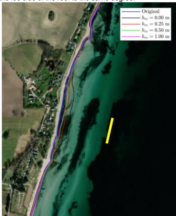
Figure 4: Satellite image including the reef (yellow rectangle), original shoreline (blue) and predicted shorelines using different h_{rc} after 9 years.
