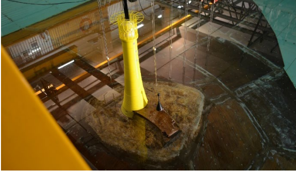
Figure 5 - Completed lighthouse model in the Ocean basin
