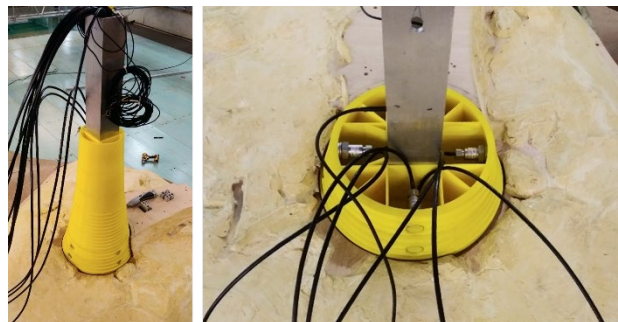
Figure 4 - Cabling for pressure transducers and load cell in the partially-completed lighthouse model
