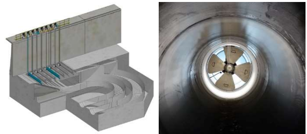
Figure 2 - Inlet/outlet structure with guiding vanes (left) and view through 2 m diameter pipe on ship thruster (right). © grbv (left); FZK (right)
