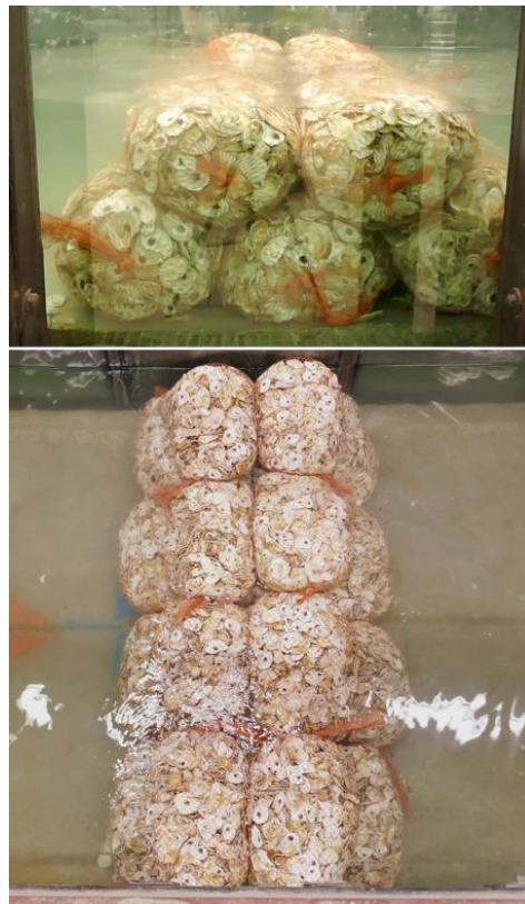
Figure 1 - Test setup of the 20 kg bags in a 5-bag berm orientation; top - view through the flume windows, bottom - view from above.
