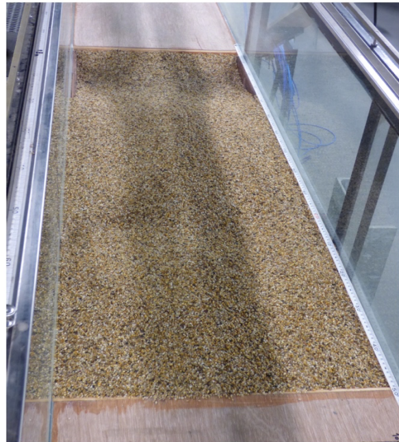
Figure 3: final bed after test with d_{50} = 3.2\text{mm} . The flow direction was from the top towards bottom of the picture.
