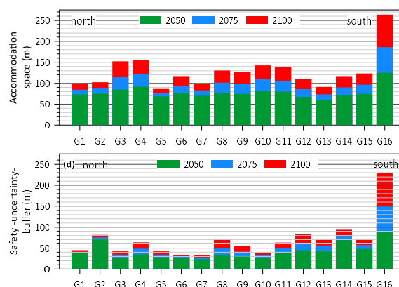
Figure 3 - Sector averaged projections of the accommodation space (top), and the safety buffer due to associated uncertainties (bottom) along the Catalan coast for different timeframes.
