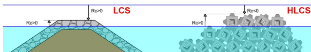
Figure 1 - Cross sections of detached breakwaters: (a) Conventional LCS, and (b) Cubipod HLCS
