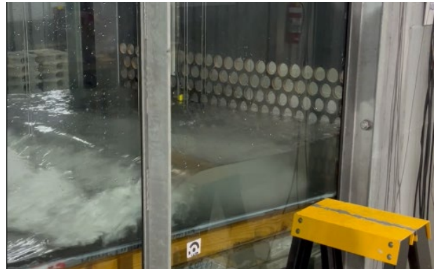
Figure 1 - Photograph of a wave passing through the perforated plywood board during the experiment with the structure placed at SWL with H_s = 0.15 m and T_p = 3 s..
