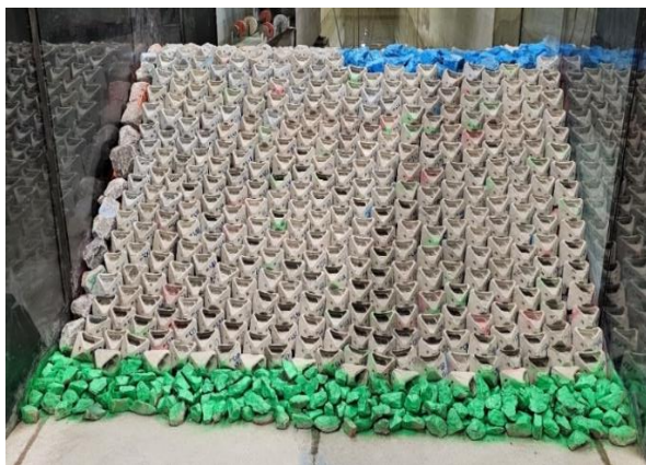
Figure 5. Conventional RMBW Model Construction
