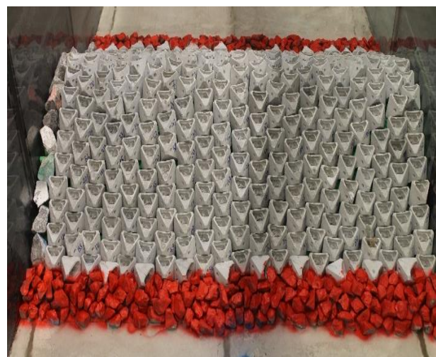
Figure 3. Low-crested Breakwater Model Construction
