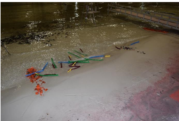
Figure 1. Model driftwood being transported onshore by breaking waves in the physical model (Murphy et al. 2020).
