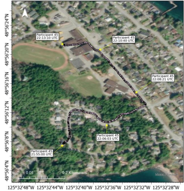
Figure 4: The GPS coordinates and UTC time recorded during the tsunami evacuation by the NEO-6M module for a 10-year-old girl (Participant ID #45).
