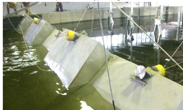
Figure 1 - Chioggia gates experimental model test of the natural period of mode 1 (1:10 scale); gates are displaced by magnets.
