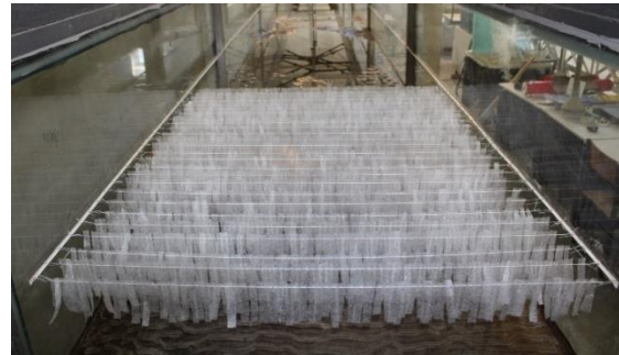
Figure 1 - Suspended offshore longline seaweed aquaculture system physical model.
