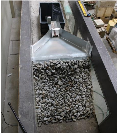
Figure 2 - Overtopping measuring set-up.
