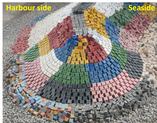
Figure 4 - Extended breakwater head section in the wave flume (Sections 0-0 and 1-1).
