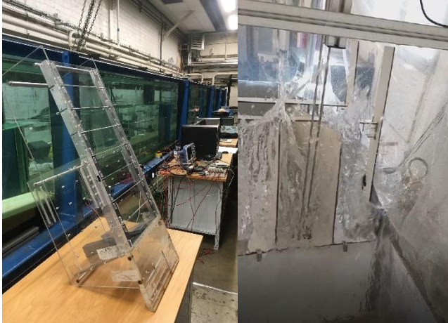
Figure 3 - Pictures of high freeboard vertical wall model in Edinburgh (left) and an overtopping event during test in Rome (right).
