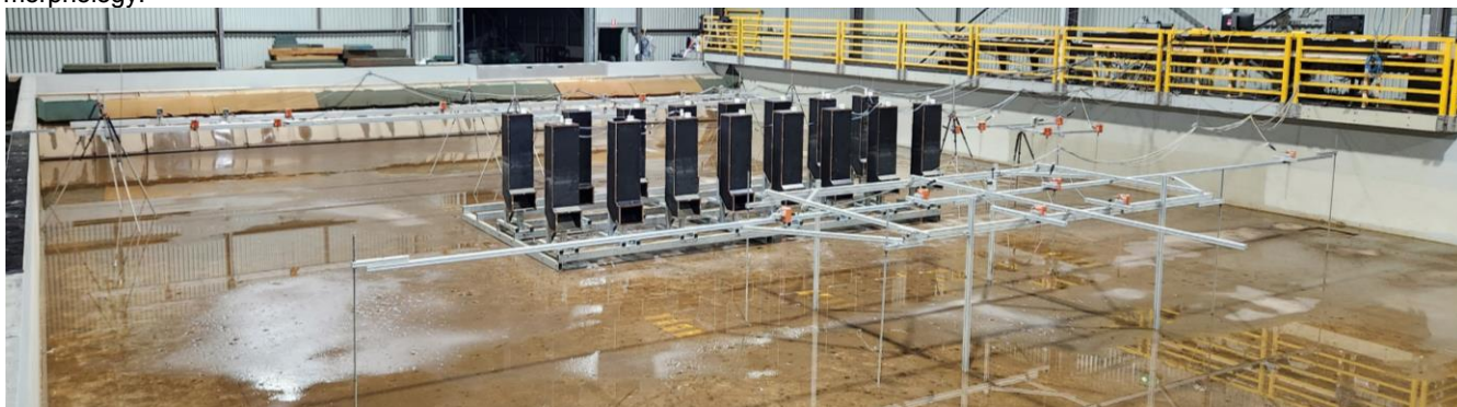
Figure 1: Array of 16 Oscillating Water Columns in the Wave Basin, arranged in two rows and equally spaced.
