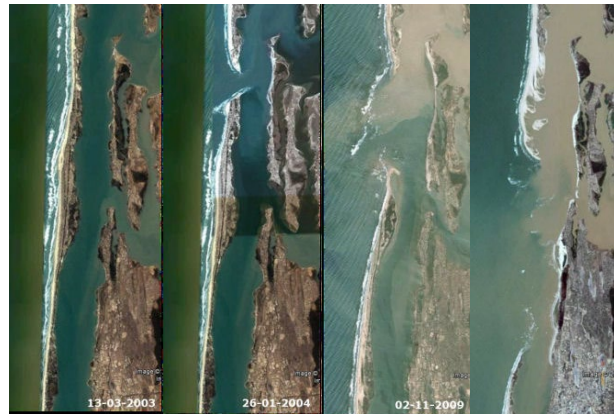
Figure 2 - The Langue de Barbarie sand spit in Senegal just before, and the years following the creation of an artificial breach in 2003 (Source: Google Earth).
