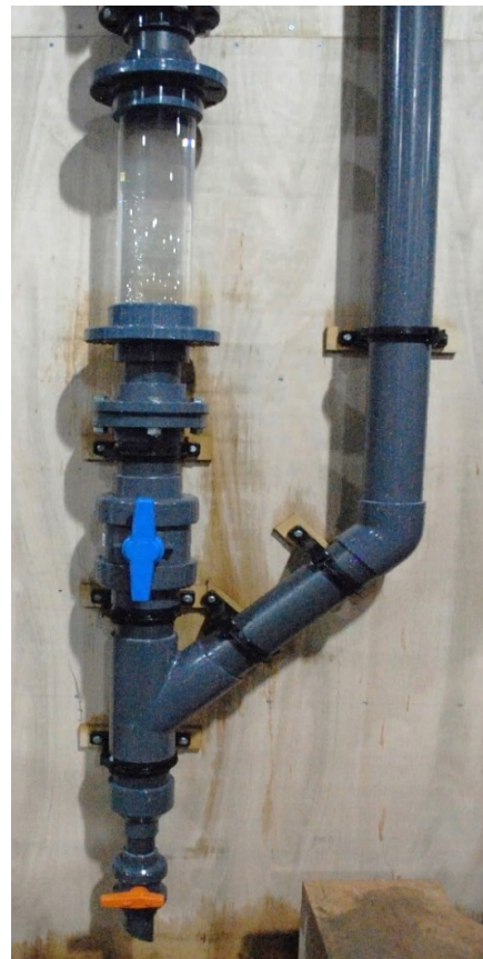
Figure 2: Oscillatory flow test rig, showing the U-tube shape and the sample container in place (clear pipe section)
